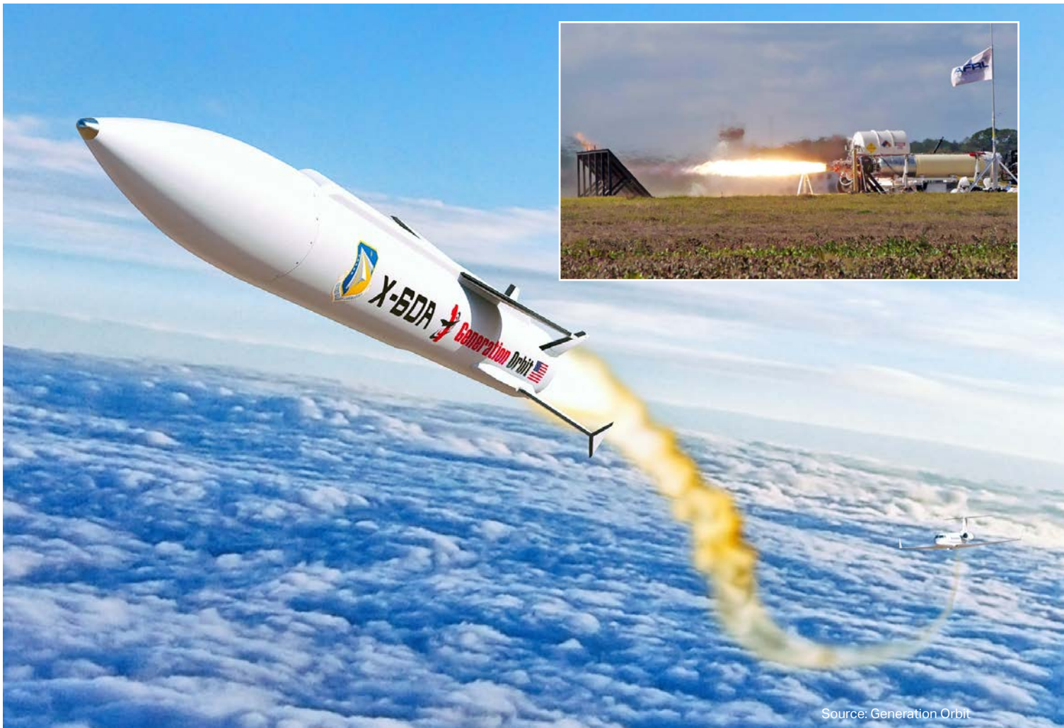
Cecil Spaceport Tenant Generation Orbit rendering of the X-60A air-launched single-stage liquid booster. Inset: Initial integrated engine firing of a full-scale, functional prototype of the GOLauncher1 (GO1) hypersonic flight test booster (June 2018).
